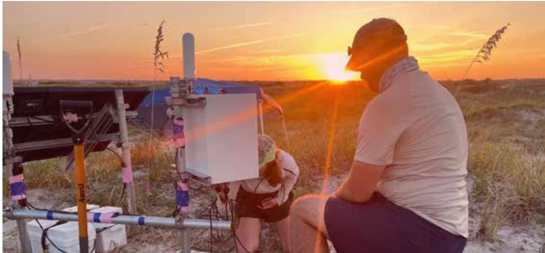
Assistant Professor Katherine Anarde , left, and postdoctoral researcher Christine Baker , right, deployed two cameras mounted on masts atop a dune at Masonboro Island, near Wilmington, North Carolina. The camera imagery can be combined to generate elevation maps of the beach from the shoreline to the dune toe. The maps will be used to examine how the beach erodes or accretes over daily to seasonal timescales. These observations can contribute to the advancement of existing models of storm impact and subsequent beach recovery. ■
