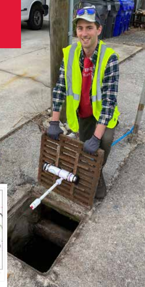
Photo of the flooded roadway during the highest observed water level on November 8, 2021. Bottom left: Measured water levels above the storm drain pressure transducer relative to the road surface. From Gold et al., (in review). Right: Thelen with a Sunny Day Flooding Sensor installed in a Carolina Beach storm drain.
