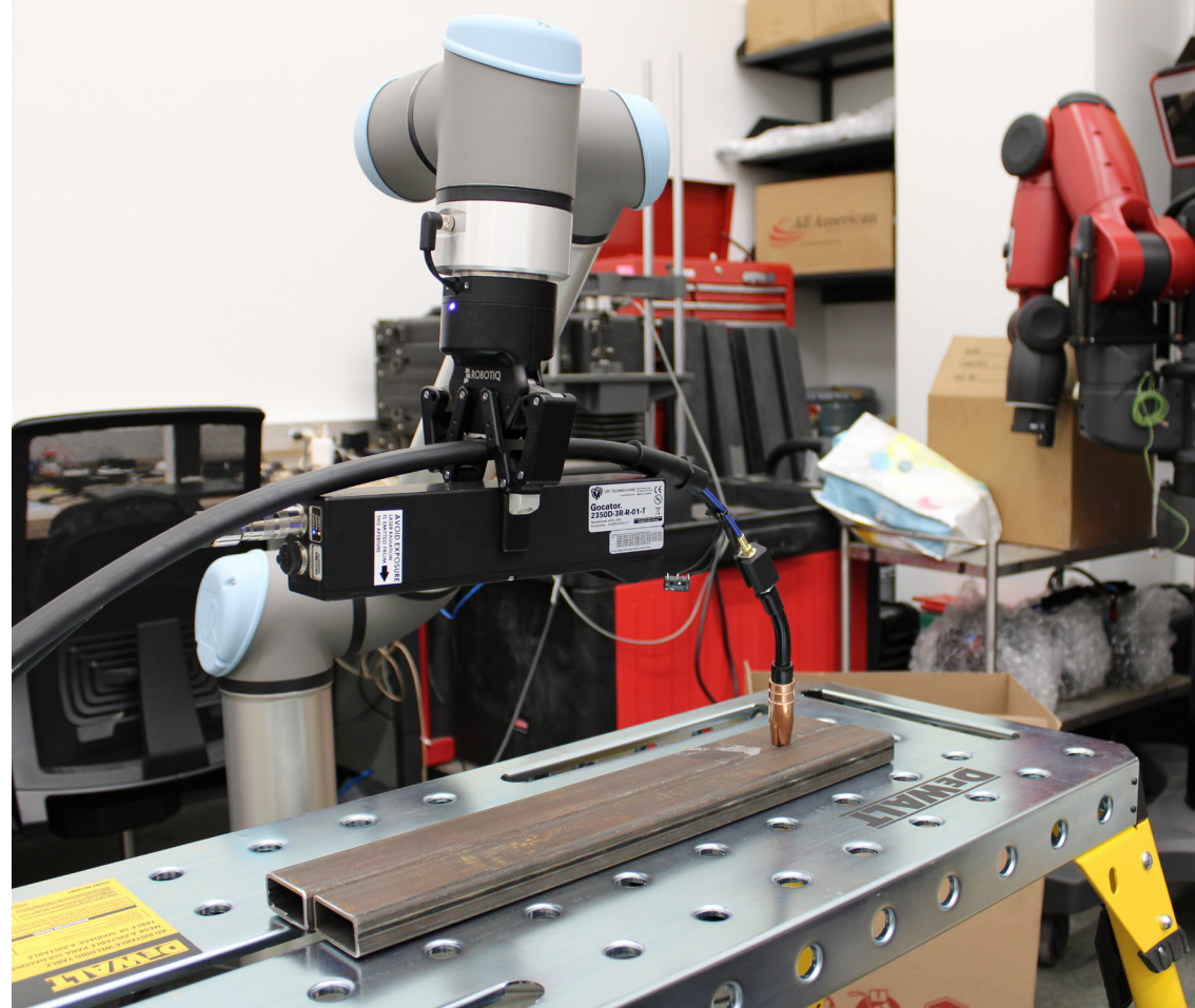
Left: Inspection robot with a terrestrial laser scanner, vertical lift and an unmanned ground vehicle with Light Detection and Ranging (LiDAR) for autonomous navigation; Right: A welding robot with a robotic arm, line laser scanner and a modified welding torch for automation.
