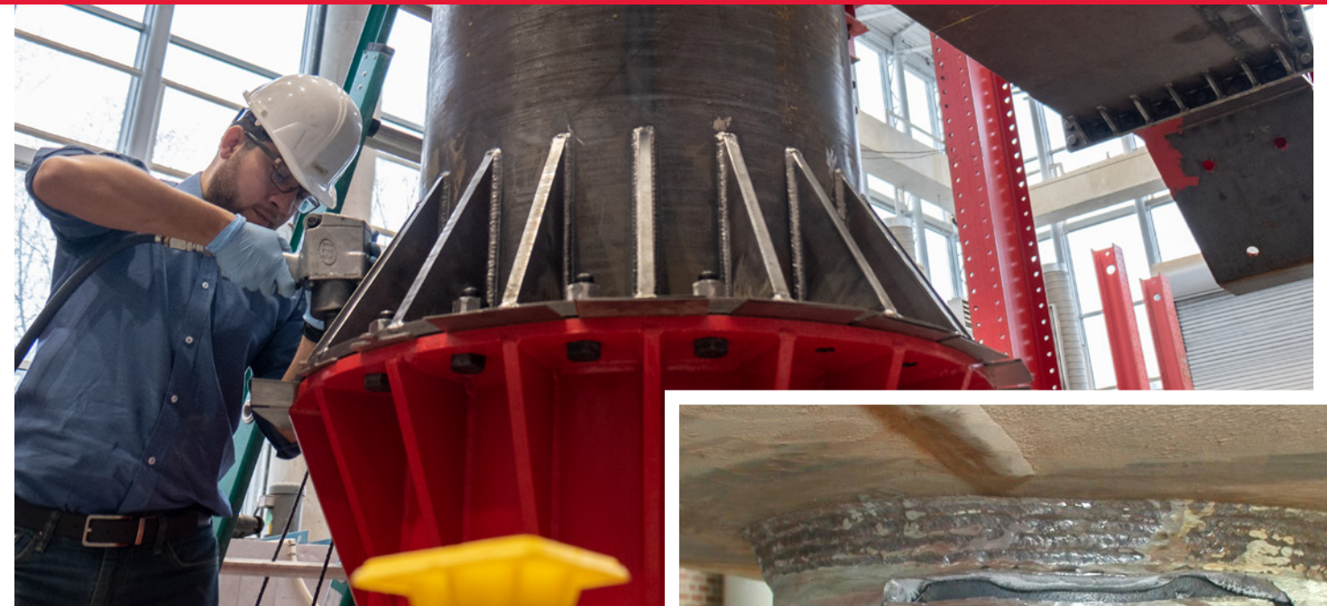
Ph.D. student Victor Calderon tightens bolts on the base of the test fixture.
