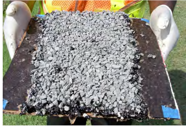
Field sample of pavement surface treatment used for performance testing
