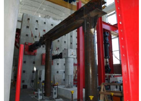
Steel Cap Beam undergoing testing at the Constructed Facilities Laboratory
