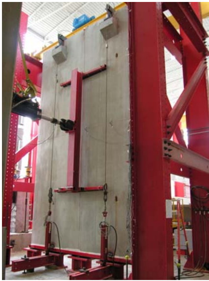
Testing of Fiber-reinforced precast concrete wall panels
