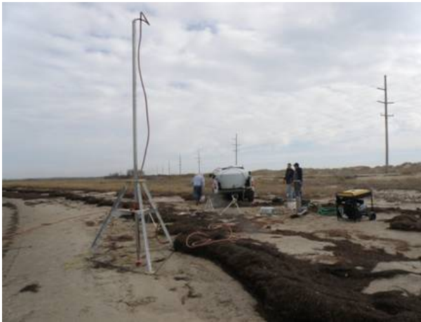
Faculty and students from the Geotechnical Engineering group use a new scour probe to test the erodability of sands near Buxton, NC. Results from these tests can be used to predict the scour potential of soils around bridge piers.
