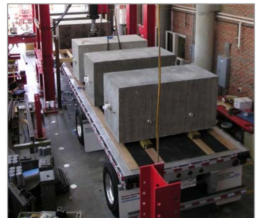
Load testing of a lightweight composite flatbed truck trailer
