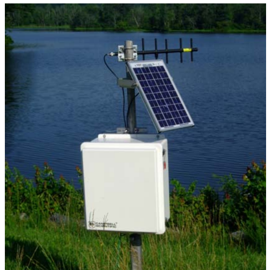
Solar-powered remote data acquisition, storage, and transmission infrastructure for a piezometer installation at Lake Raleigh Dam.
