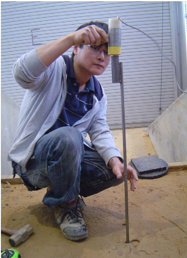
Sangchul Pyo and Brent Robinson (not pictured) apply seismic wave to the subgrade to estimate shear modulus.
