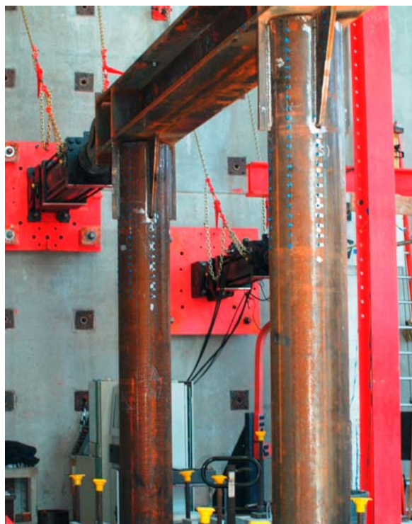
Seismic Testing of Steel Bridge Bent for Alaska DOT
