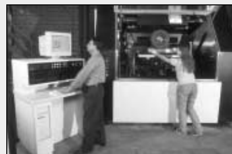
The Automated Wheel-Track Pavement Testing System being used by Paul Khosla and several graduate students was obtained under the recent NSF Equipment Grant.
