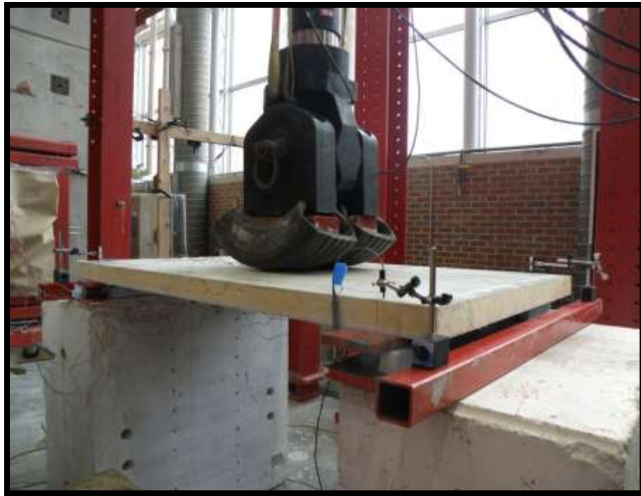
Typical test setup evaluating two way flexural behavior
